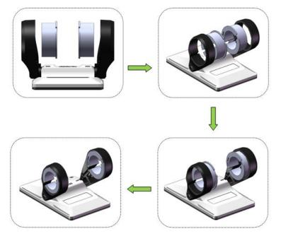
Note: The installation direction of the adjusting washer must be from the inside to the outside of the bracket.
